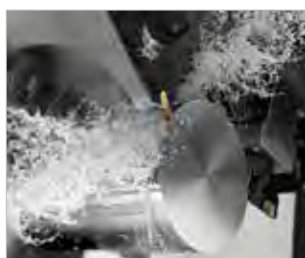
Standard Coolant (Nozzle)
