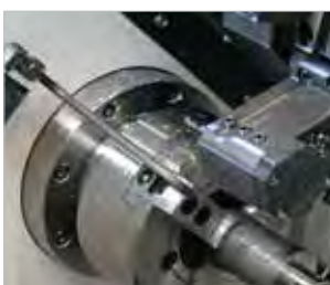
Chuck Air Blow (Upper Chuck)
